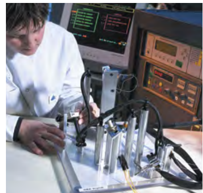
AUTOMATIC CONTINUITY AND INSULATION TESTING
